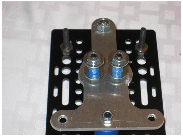
The eccentric spacers have a mark on them that indicates where the narrowest point of the offset is located. Set this mark to the top of the gantry plate for now. There are several models of eccentric spacer, yours may have a Line notch instead of an imprint.
