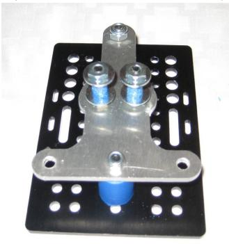
**Step 11:** Assemble all 4 Openbuilds wheels by installing the two included bearings into the wheels, one per side. They should snap into the housing, and sit flush with the edge of the wheel.
