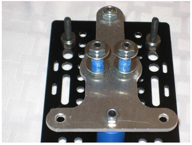
Step 15: Install the wheel assemblies on each bolt
