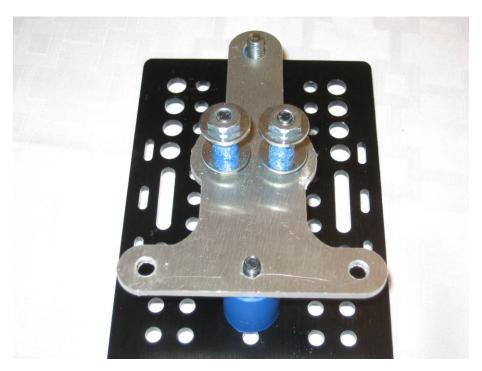
**Step 10:** Secure the M6 and M6 nuts to lock the backplate in place.
