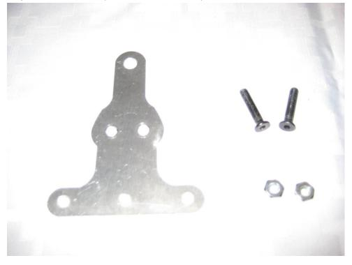
**Step 6:** Insert the bolts through the back of the backplate, then install the nuts. Tighten the nuts down until they are very tight.
