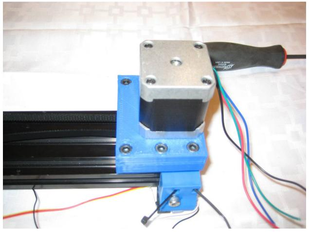
**Step 48:** Attach the other side of the belt to the posts. Trim any remaining excess belt or zip tie ends. You will tension the belt later once the assembly is bolted to the Taz.
