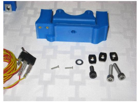
**Step 32:** Insert the 20mm M5 bolts through the top and bottom of the Idler endcap, and the 10mm M5 bolt and washer through the front. Preinstall the M5 Tslot nuts on those bolts. Optionally, install the X maximum Endstop with the 8mm long M2 bolts. Set aside, along with the 2 32mm long M5 bolts and the
