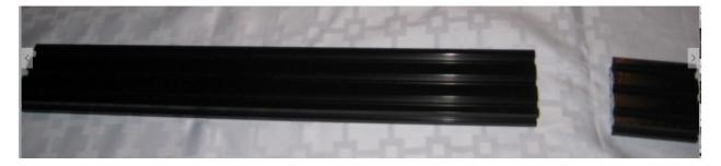
Measure your 500mm x 60mm x 20mm Openbuilds rail to ensure it is in fact actually 500mm long. If so, remove 64mm using a metal blade hacksaw and a miter box. The openbuilds X axis design allows for approximately +/- 2mm error on this cut.
