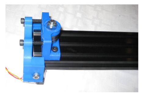
**Step 46: (Optional)** If you installed the X maximum endstop, route the endstop cable through the Openbuilds rail as shown and out the other side, where it will join the X minimum endstop cable path.
