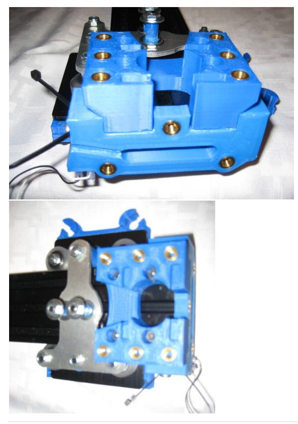
**Step 42:** Check for clearance of the X carriage on both sides, and alignment with the endstop.
