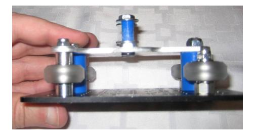
**Step 22:** Locate the **Taz\_Openbuild\_X\_Carriage\_1\_2\_a.stl plate**, the stock Taz 4/5 Carriage guide, and the stock 4 m3 10mm bolts and washers
