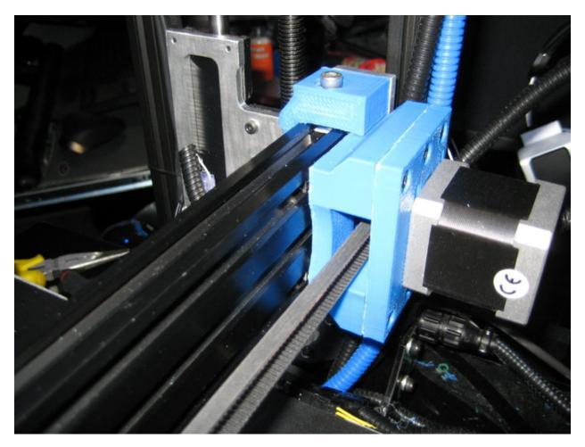
**Step 50**: tighten the idler tension bolts until the belt makes a tone when plucked top and bottom. Once the idler is in place, tighten the rail side bolts to ensure it doesn't move. Use zip ties to secure the extruder wire harness cable(s).
