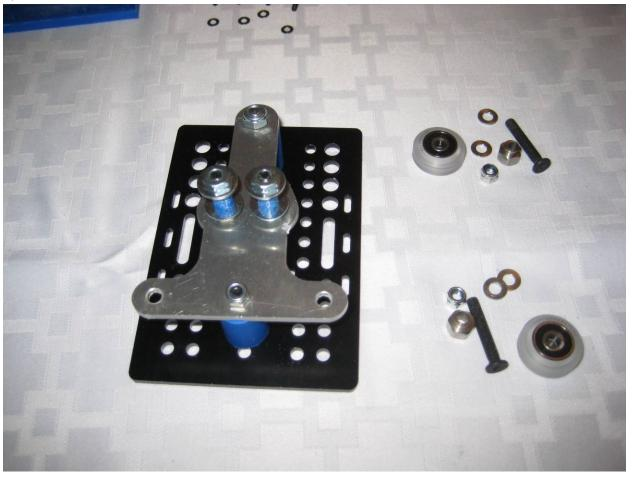
**Step 13:** Insert the M5 bolts through the gantry plate in the two outer 2.2mm holes, one row down from the top (as shown in the picture). Insert the Eccentric spacers so that the smaller section sockets into the 7.2mm hole surrounding the bolt.
