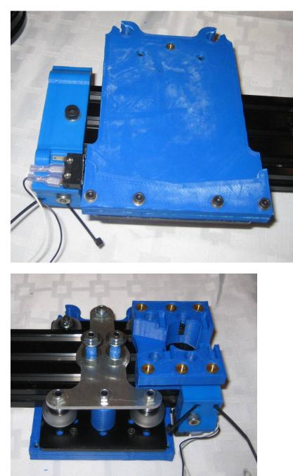
**Step 43:** Loosely slide the X idler block onto the openbuilds rail, do not tighten it at this time.
