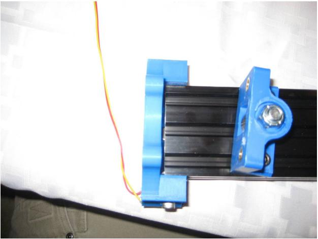
**Step 45:** Install the M5 32mm long bolts through the idler endcap and into the idler block. Tighten them until they bottom out, then back them each off 4 turns. These bolts will allow you to adjust the belt tension on your X axis belt.
