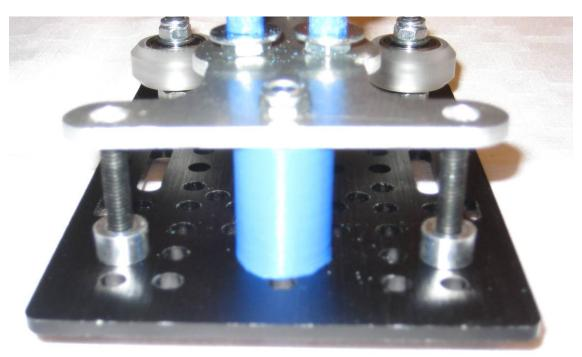
Step 19: Slip one of the 6mm non eccentric spacers over each bolt
