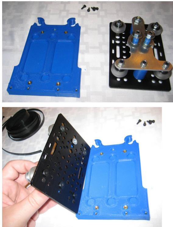
**Step 24:** Flip the adaptor plate over, locate the 4 8mm M3 screws, and position the X carriage gantry plate and back plate assembly so that the bolt heads line up with the recessed cirles
