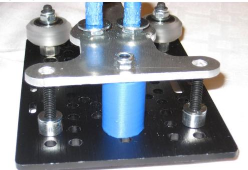
**Step 21:** Slip another washer, the other spacer over each bolt, extend the bolt through the backplate, then add the M5 lock nut. Yes, I skipped a couple of pictures. Sorry.
