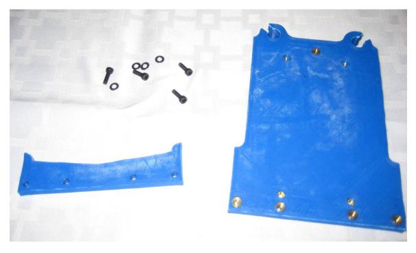
**Step 23:** Install the carriage guide to the adaptor plate, ensure that the notch slopes down towards the plate so that it mirrors the stock configuration
