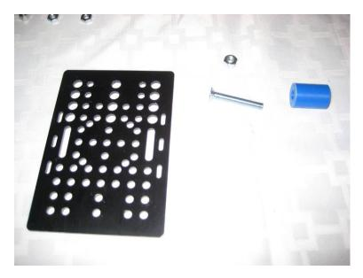
**Step 2:** Insert the M6 35mm bolt through the second from the top 7.2mm center hole in the gantry plate as shown in the picture, then install the spacer.
