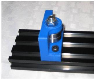
**Step 44:** loosely install the Idler endcap onto the rail. You will want an approximate 5mm gap between the end of the rail and the inner wall of the endcap as shown below. This will allow for adjustment when the rail is installed on your Taz and is by design. You will tighten the bolts later once you install the rail into your Taz
