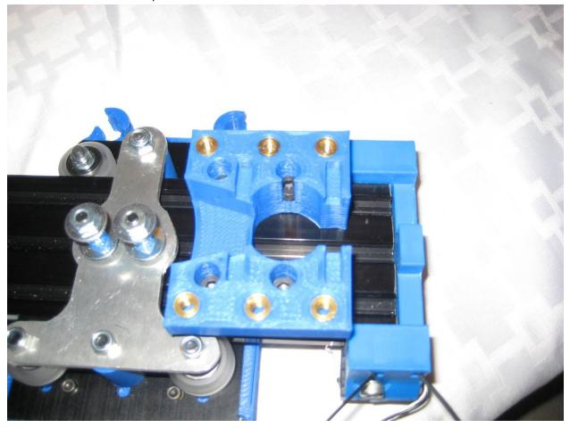
**Step 41:** Slide the X motor main block over so it is flush with the outer edge of the X motor endcap. And tighten all of the bolts.
