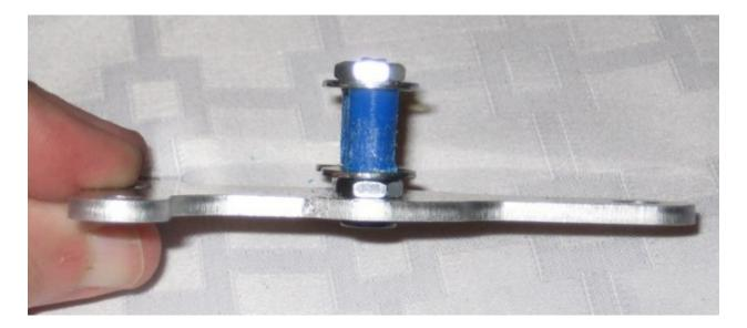
**Step 9:** Place the assembled backplate on the Gantry plate assembly as shown in the picture:
