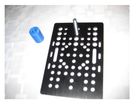
Step 3: Locate the flat head 35mm M5 bolt and nut and the Taz\_Openbuild\_X\_bottom\_backplate\_spacer.stl
