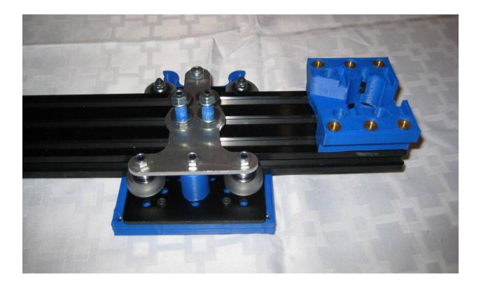
**Step 40:** Install the X motor endcap as shown. Ensure that there is no gap between the end of the rail and the inside of the endcap.
