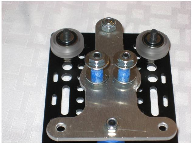
**Step 17:** Install the locknuts. Tighten them until the wheel has no wobble or play on the bolt, but still moves freely. If the wheel seems difficult to turn or has drag, back the nut off a small amount until it turns freely again.
