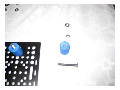
**Step 4:** insert the 35mm bolt through the second from the bottom 5.2mm hole in the gantry plate and then install the spacer (Not pictured)
