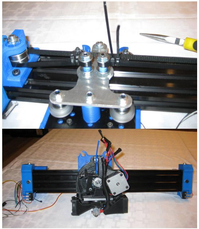
The Completed open builds assembly, with a toolhead mounted.
