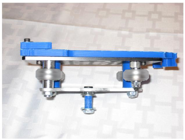
side view of the completed X carriage Assembly
