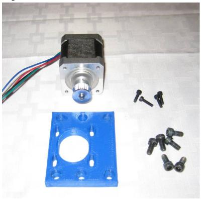
**Step 34:** Install the motor using the 4 M3 bolts. It is adjustable later. Preinstall the 6 M5 bolts so they are flush with the recessed sockets. Set the completed assembly aside for later. **Note:** You can use a vibration damper here if you like, however the design of the mount already serves that purpose so there is no real gain to doing so at this location.
