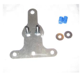
**Step 8:** Install a second set of 2 washers and 2 nuts on the bolts, tighten. You may optionally apply blue Loctite to the last bolts.
