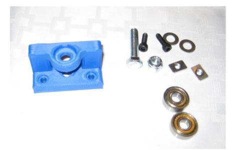
**Step 29:** Reinstall the stock Taz idler hardware, with the bolt head at the bottom of the idler block, followed by a washer, 2 608zz bearings, another washer, and then the Nut on the outside of the assembly as shown in the picture below.
